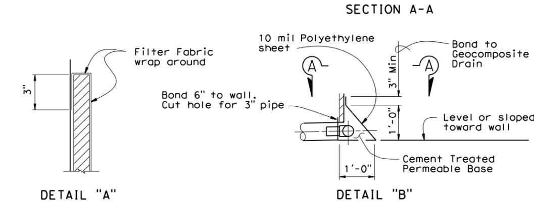
**WEEP HOLE AND GEOCOMPOSITE DRAIN**
